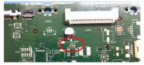
Note that the AL fuse is NOT located near the AL connector (see following picture)!
